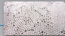
Zirconia beads installed in inner casing
