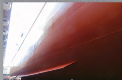
Condition after applying 2nd coat of X-mile (AF)
