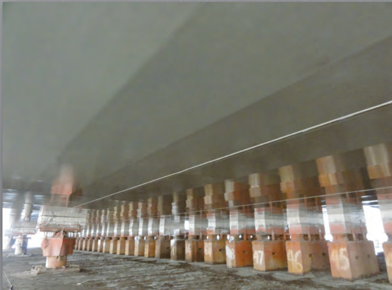
Condition after applying X-mile AC & Surfacer (Reflecting wood block on paint film surface)
